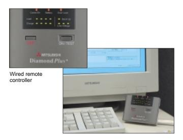
Removable wired monitoring and controller unit allows the user to perform UPS ON/OFF operations and status monitoring at close proximity on desktop. Quick glance at the display allows the operator to react quickly to any situation that may present itself and perform any corrective actions to prevent any potential data loss.
