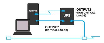
UPS backup power during commercial power failures can be separated into two systems via the output load receptacles. In cases where several kinds of equipment are connected, the load shedding function allows the UPS to deactivate backup support for peripherals and allocate battery power on a priority basis to critical equipment that needs to perform shutdown operations.
